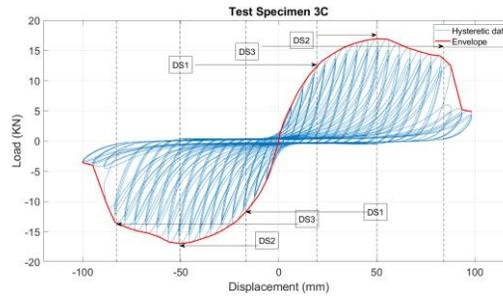
Figure 1. Example of damage states for a test specimen; test data from Boudreault (2005).
