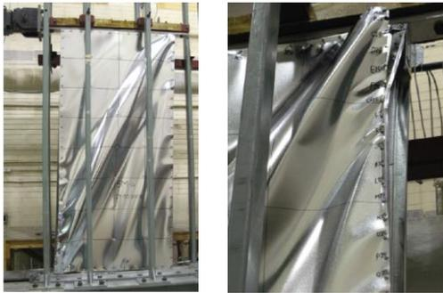
Figure 5. DS3 example for walls with steel sheet sheathing (a) buckling of steel sheet; (b) Twisting of stud (image: [6])
