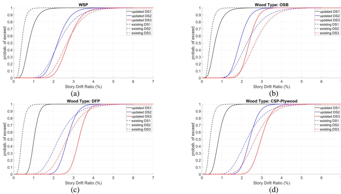
Figure 4. Fragility curves for CFS walls with WSP sheathing: (a) all; (b) OSB; (c) DFP; (d) CSP or Plywood.
