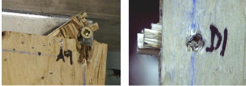
Figure 2. Examples for failure of walls with WSP sheathing (corresponding to DS3):
