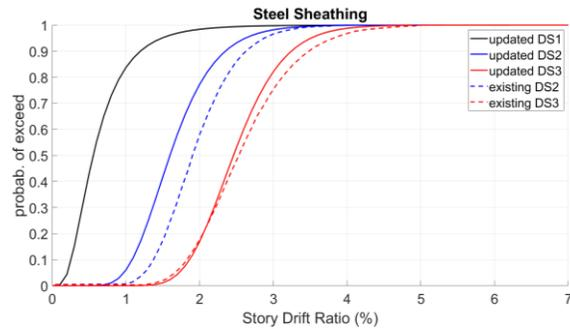
Figure 6. Fragility curves for all CFS walls with steel sheet sheathing.
